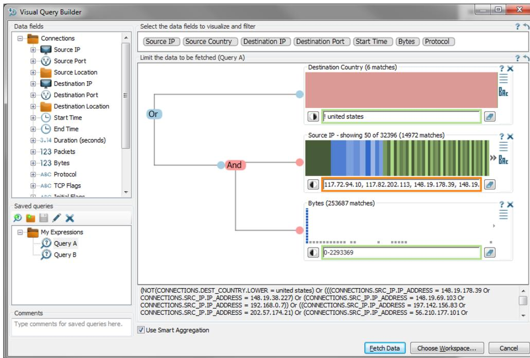
**Figure 1.** Our visual query builder, showing a request for Source IP, Source Country, Destination IP, Destination Port, Start Time, Bytes, and Protocol for records destined for outside the United States or records matching a short list of source IP addresses and having a bytes value between 0 and 2,293,369.
