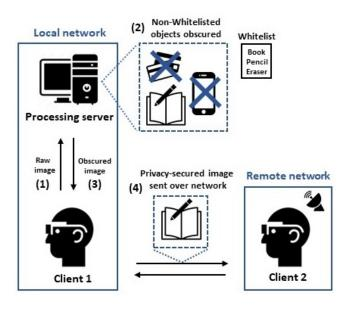
Figure 1: Architectural overview of Erebus and its four main steps
